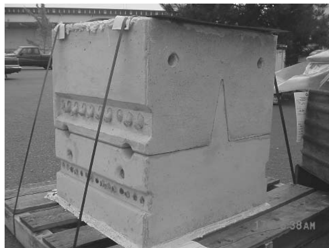
Fig. 5 A matched ceramic die set for hot sizing of titanium 6Al-4V. The die set is 1 × 0.75 × 1.5 m high.
