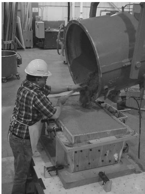
Fig. 9 Pouring of the raw ceramic into a casting mold
