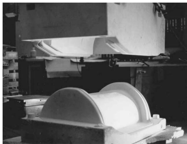
Fig. 4 SPF ceramic die set with preform ribs around the periphery and indexing nubbins. The die halves are approximately 1 × 1.5 × 0.5 m high.
